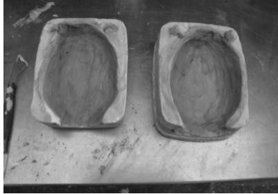
Picture 3: The two half parts of the plaster mould
