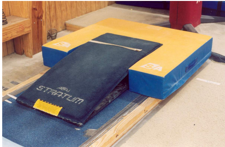
FIGURE 1. Vault board with a line taped at the peak of the vault board’s upper section curvature.
