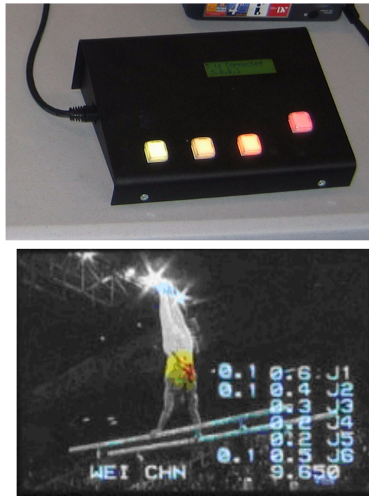
FIGURE 7. Box for judges and recording on video the deductions of judges (Čuk, Forbes, 2006)
